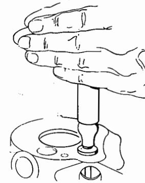
Handlapping a valve and seat
