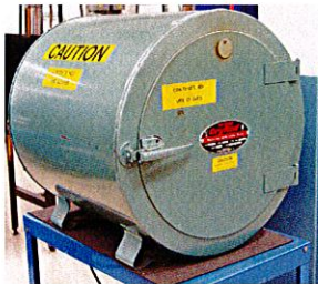
Figure 34 – Stationary Electrode Storage Oven
