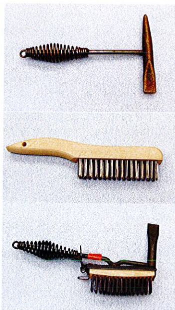
Figure 29 – Chipping Hammer, Wire Brush, and a Combination
