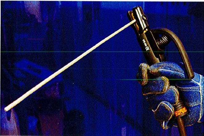
Figure 25 – Clamp Style Electrode Holder
