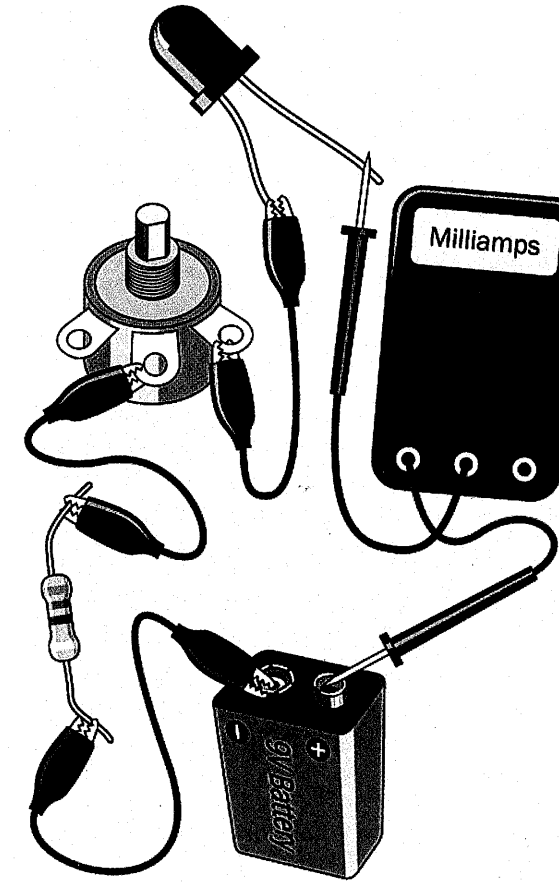
Figure 1-56 The current flowing through a simple circuit is always the same throughout the circuit, regardless of where you measure it.
