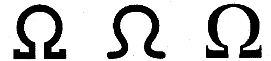
Figure 1-6 Three samples of the Greek symbol omega, used to represent electrical resistance.
