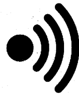
Figure 1-7 This symbol indicates the option to test a circuit for continuity, with audible feedback. It's a very useful feature.
